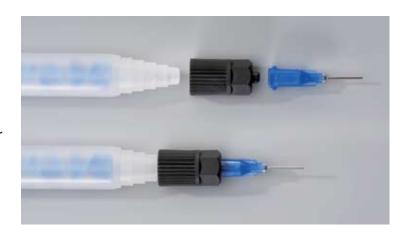
Luer Lock Adapters are available in a variety of sizes to fit static mixers ranging from 5mm to 10 mm outer diameters. They attach firmly and securely to the mixer and possess a universally sized outlet on the opposing end to easily adapt to whip hoses, needles, reducers and other commonly utilized fittings.
